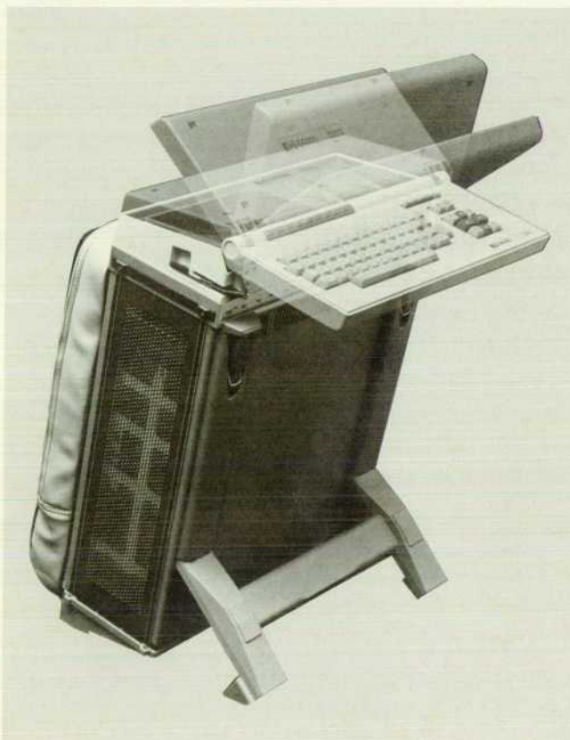
Fig. 1. The 64110A Development Station is designed for easy transportability and can be hand carried or moved on a typical luggage dolly. The 64110A can be set on a bench, rack mounted, or set on the floor steadied by its rear feet as shown. The keyboard can be adjusted to a convenient work position and an optional pouch can be mounted on top of the 64110A to carry cables, connectors, and pods.
