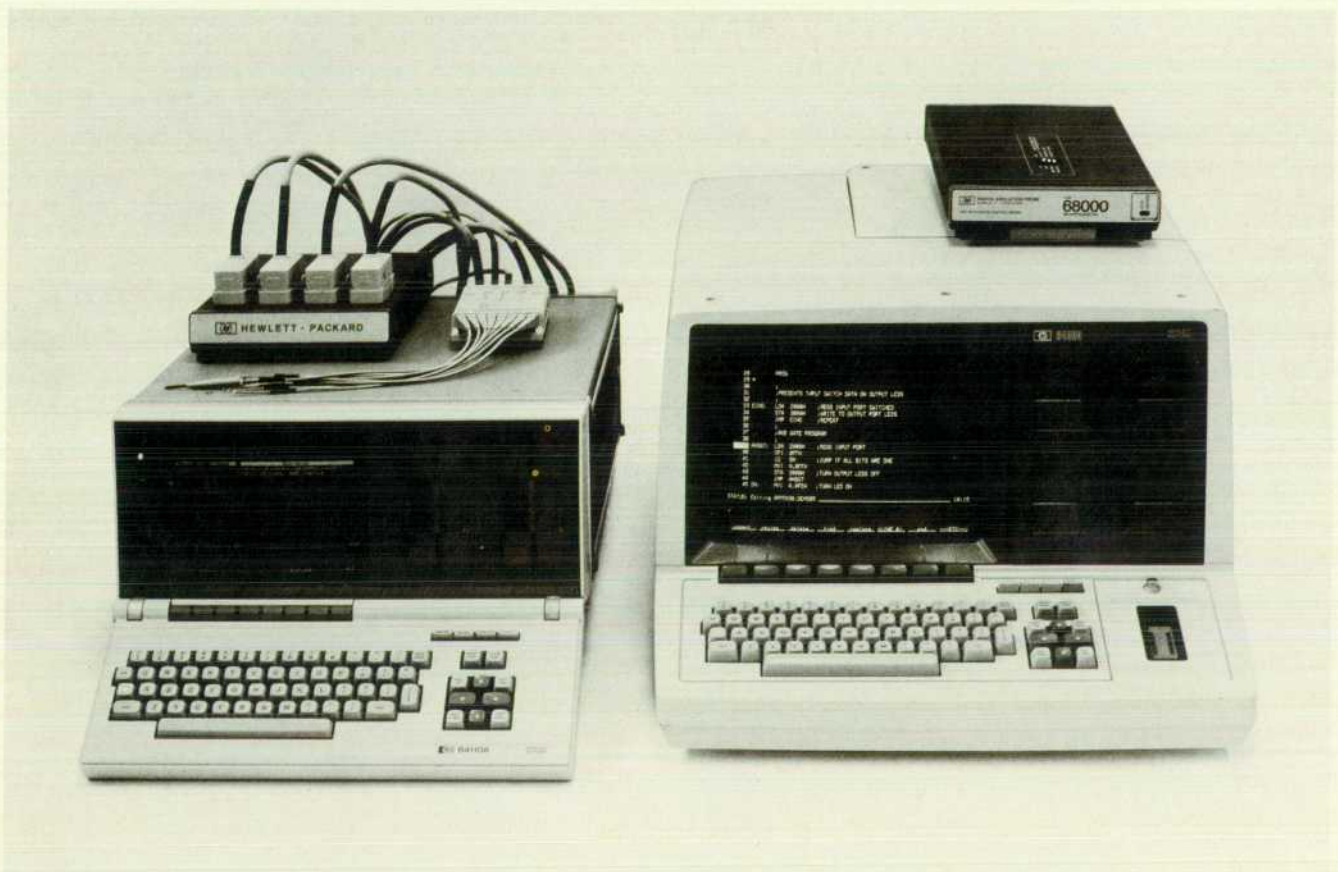
Fig. 1. The HP 64100A Development Station (right) includes a keyboard, display, host processor, space for 10 option cards, dual flexible disc drives, and power supply. The optional emulator for the 68000 microprocessor is shown on top of the 64100A. The HP 64110A Development Station (left) is the transportable version of the 64100A and has the same features except that the number of option cards is limited to five. Some of the cables and a pod for the HP 64620S Logic State/Software Analyzer option are shown with the 64110A.
